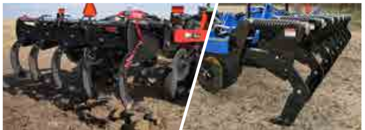
Parabolic shanks with hydraulic trip
