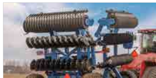
DOUBLE V BLADES NOTCHED FRONT, SMOOTH BACK
