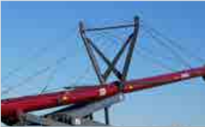
CABLE TRUSS SYSTEM
