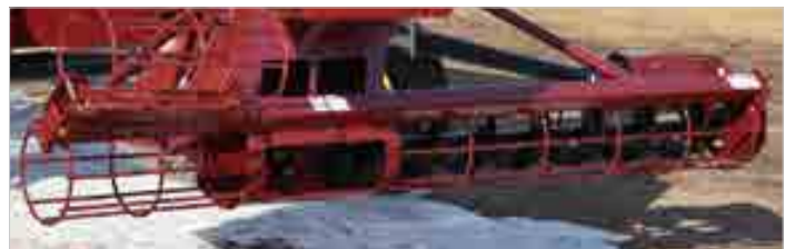
9" CROSS AUGER WITH CONTINUOUS FLIGHTING
